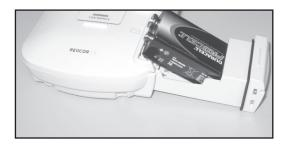
Close the drawer and press the blue slider down until it snaps in place with an audible click.
