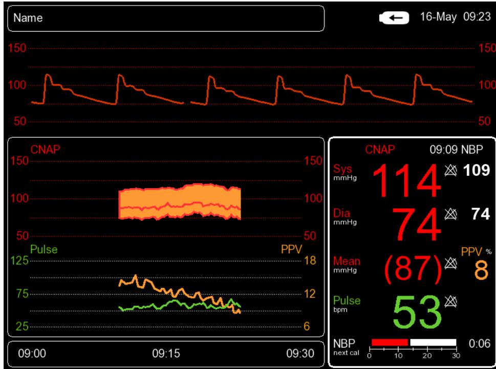
**Illustration 48: Display of the CNAP™-PPV during a measurement**
