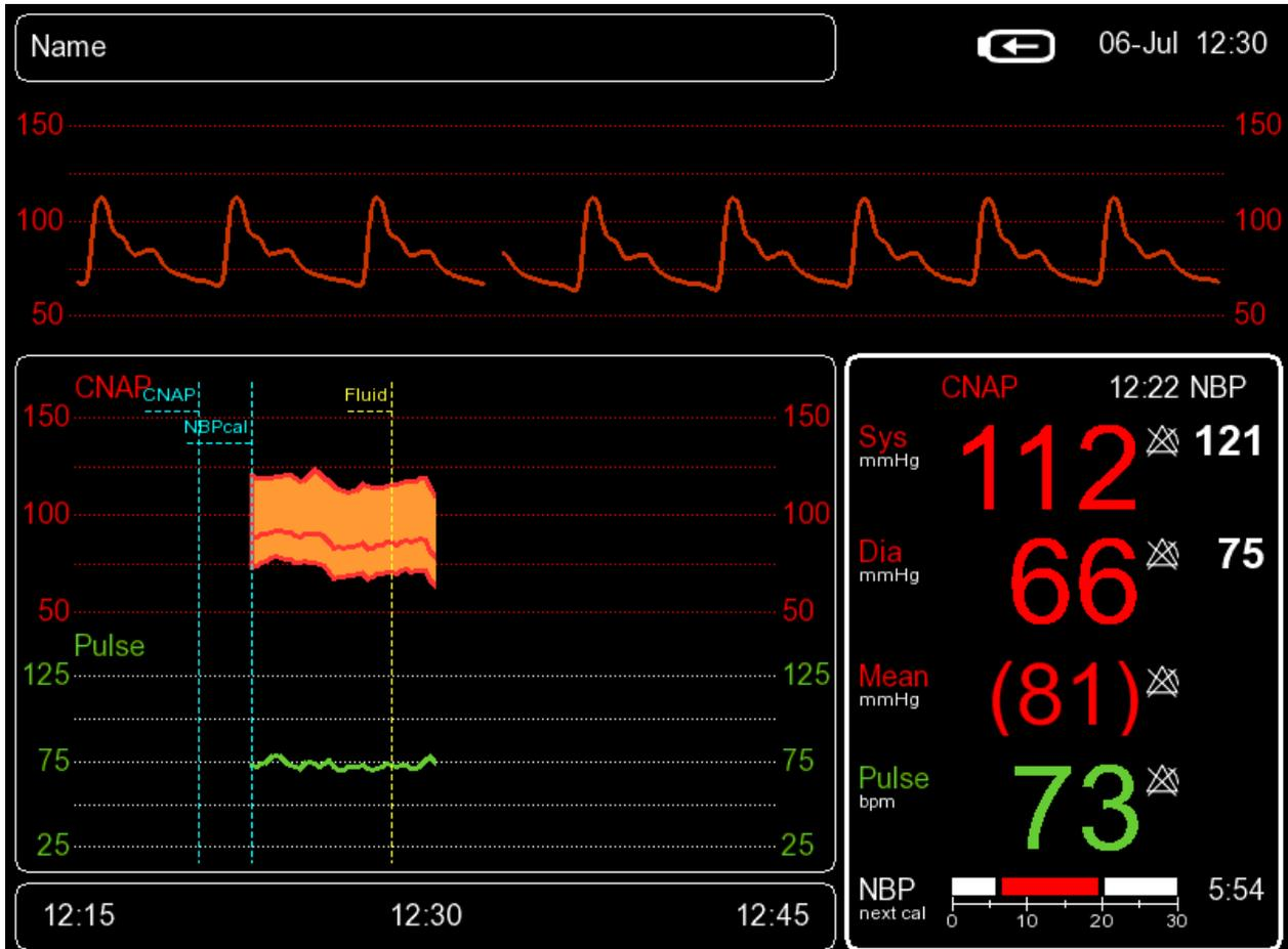
**Illustration 32: Automatic and manual interventions during a CNAP™ measurement**
